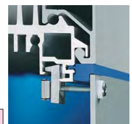
Spacer trim For installed equipment flush with the frame section. For front panel thickness up to approx. 0.14" (3.5 mm).
